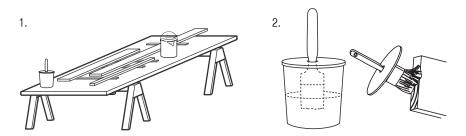
1. Set up a priming station at the jobsite
