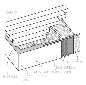
RAINSCREEN ON TOP OF HOUSE WRAP WITH BUG SCREEN AT BOTTOM OF JOIST.
