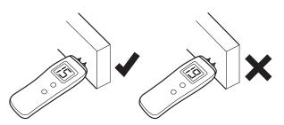
**NEVER ABOVE 18% MOISTURE:** Before installation, ensure that the WindsorONE Trim Boards are dry. Do not install Trim that has a moisture content above 18%. (See page 5 for more on moisture content.)
