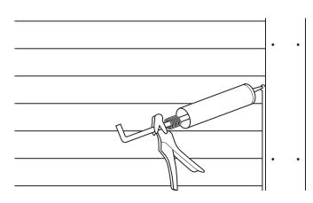
**TYPE:** Use exterior grade high-performance acrylic-latex, silicone, acrylic, or urethane caulks and sealants to seal gaps around windows, doors, corners, and other exterior joints that are exposed to potential water intrusion.
