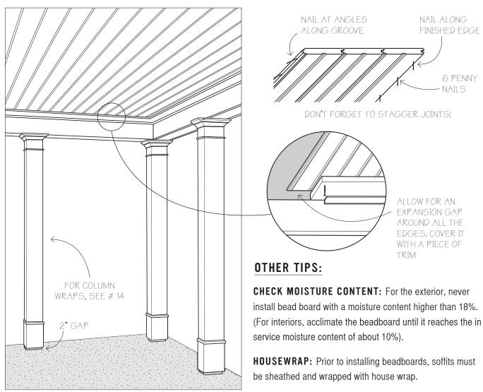
**Always isolate beadboard** from framing members and soffit/attic spaces. Moisture and humidity and any water intrusion will alter the moisture content of beadboard and could radically affect the installation.
