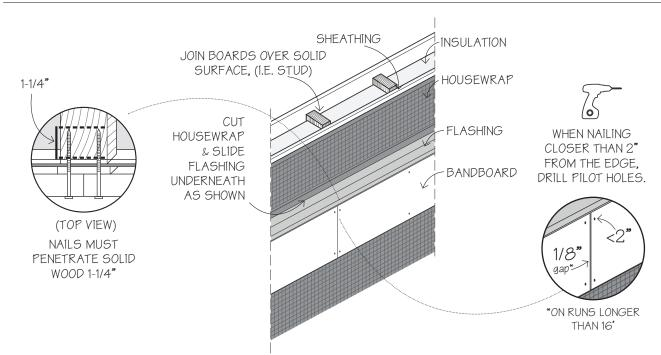
**Joints over framing.** All joints where two pieces meet end to end must occur over framing. Butt joints are recommended for both horizontal and vertical trim. In runs of 16' or less, the ends should lightly touch. Runs over 16 feet
