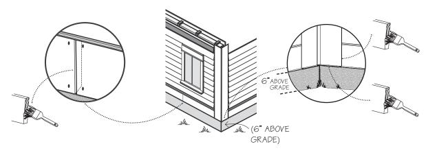
All cuts must be reprimed. Prior to installation, all trim board surfaces exposed by jobsite field cuts must be reprimed. In wet climates, also treat field cuts with a paintable water repellent preservative and a latex top coat.
