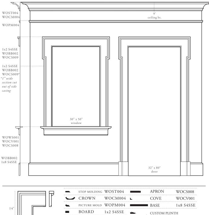
1x3 S4SSE (8-1/2"length) with bevel & 5/4x10 S4SSE trimmed from 1-1/16"x 9-1/4" to 1-1/16"x8-1/2" (6" length)
